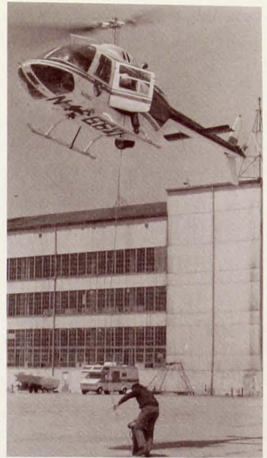
The aerial rescue rope (left) developed by Sgt. Carl Marshall is now mandatory equipment on all Maryland State Police Bell Jet Rangers. The harness on the device provides a quick way to pick up victims and move them to a safe area nearby. Training in the use of the rope (right) is now an integral part of the aviation program.
