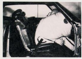
An airbag is located in the dashboard or steering column of a car. In a front-end collision, the airbag inflates instantly to prevent the driver and passengers from hitting the windshield or dashboard. It inflates and deflates so rapidly that people involved in accidents are hardly aware it has operated. (Photo courtesy of U.S. Department of Transportation)
