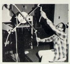
Conrad Yung-Kwai, industrial science specialist, demonstrates the BTE Work Simulator with an attachment requiring overhead reaching and grasping. This simulates a job pulling rope or cable.
