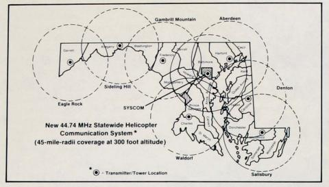
The new 44.74 MHz frequency communications system uses eight transmitters/towers to give SYSCOM contact with every MSP Med-Evac helicopter in the state.
