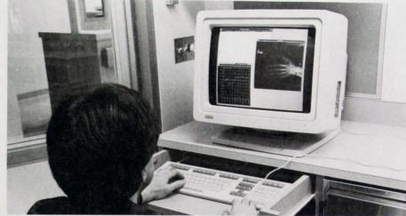
Bedside workstations have a variety of processing, windowing, and graphics capabilities. These powerful units will store patient data, which will be "dumped" to permanent storage in the computer center at planned intervals.
