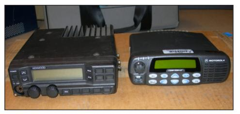
Acceptable narrowband-capable mobile radios are the Kenwood TK 890 (the KCH-11 model is shown) (left) and the Motorola Model CDM 1550 (right). Please note that the only mobile radio reimbursable under the Radio Grant Program is the Motorola Model CDM 1550.
