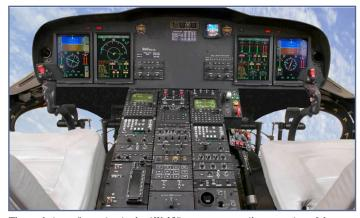
The cockpit configuration in the AW-139 supports two-pilot operation of the aircraft.
