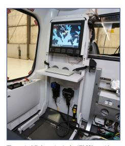
The tactical flight station in the AW-139 provides a searchable database with the ability to identify any location or address and links to the Wescam MX-15i camera, TrakkaBeam 800A search light, and flight management system (autopilot) for aircraft navigation.
