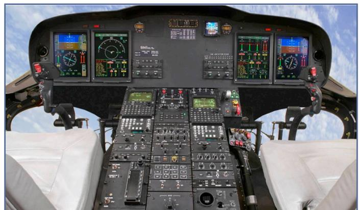
*The cockpit configuration in the AW-139 supports two-pilot operation of the aircraft.*
